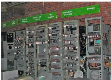
Manchester Baby, also called the Small-Scale Experimental Machine (SSEM) University of Manchester, UK, 1948. Considered 1st electronic stored-program computer.
