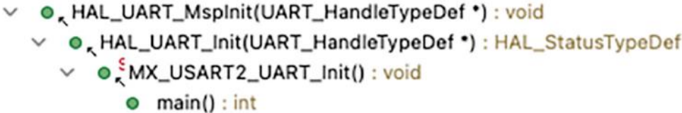
Figure 4.16: The Call Hierarchy of the function HAL_UART_MspInit()
