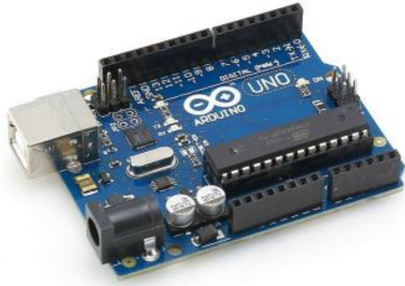
Figure 1: The hugely popular Arduino Uno board is used as the microcontroller platform of choice in the EECE module.
