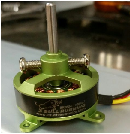
Fig. 13: Picture of the Bull Running motor modeled in our simulations and used in the hardware testing.
