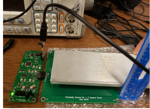
Fig. 5. Experimental setup for testing the detection of metal targets approaching the proximity sensor.
