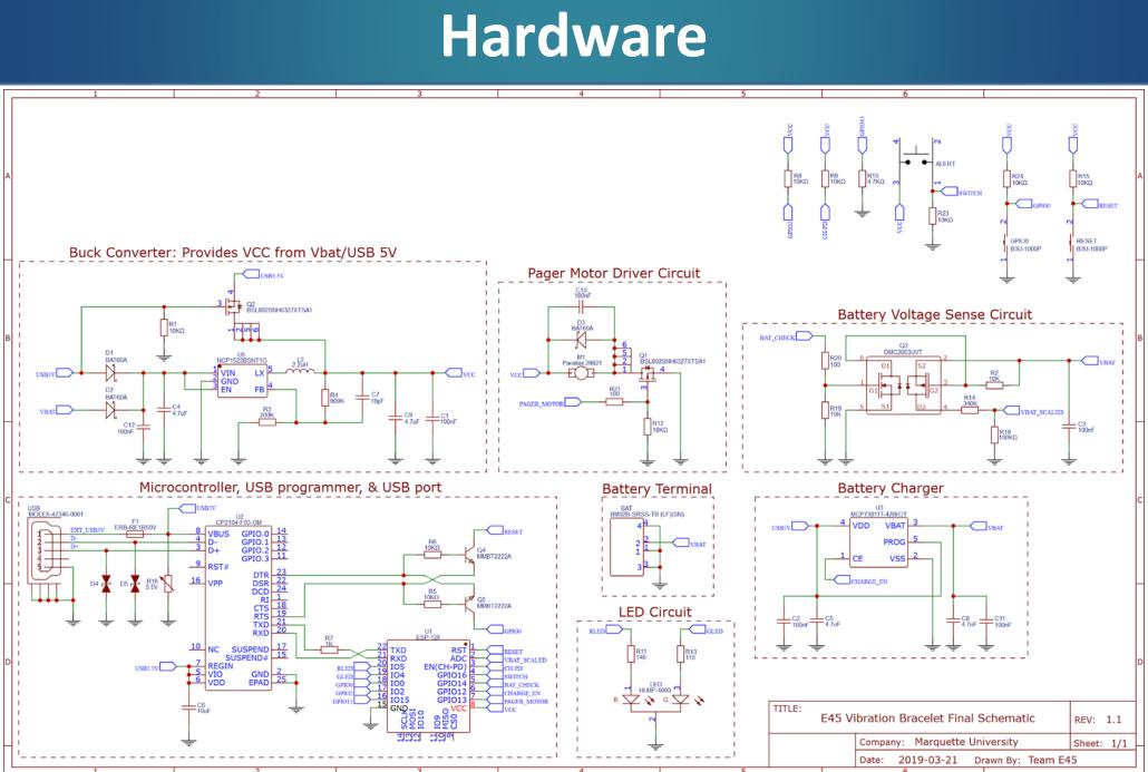
The hardware implementation is centered around an ESP8266 microcontroller. The ESP8266 was chosen for its integrated WiFi radio, low power operation, and wealth of open-source code libraries.
