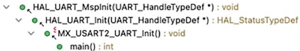
Figure 4.16: The Call Hierarchy of the function HAL_UART_MspInit()
