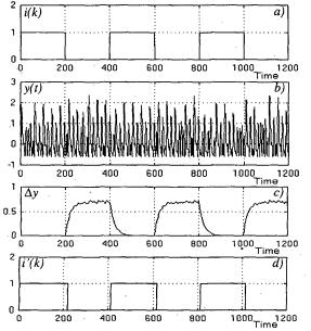
Fig.4 Waveforms of the transmitted information signal a), the transmittec chaotic signal b), the error signal at the receiver c), and the recovered signal d)
