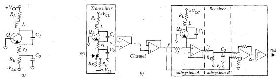
Fig.3 Block diagram of the modified Colpitts oscillator a) and block diagram of the transmitter-receiver system b)
