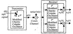
Fig. 2 Diagram of the communication system using chaotic switching
