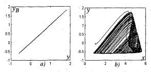
Fig.5 Chaotic synchronization of the transmitter and the receiver a) and state space trajectory projection on the plane y-x at the transmitter b)
