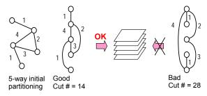
Figure 3 Illustration of good and bad initial linear placement of partitions into layers
