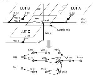
Figure 7 Illustration of the routing graph construction
