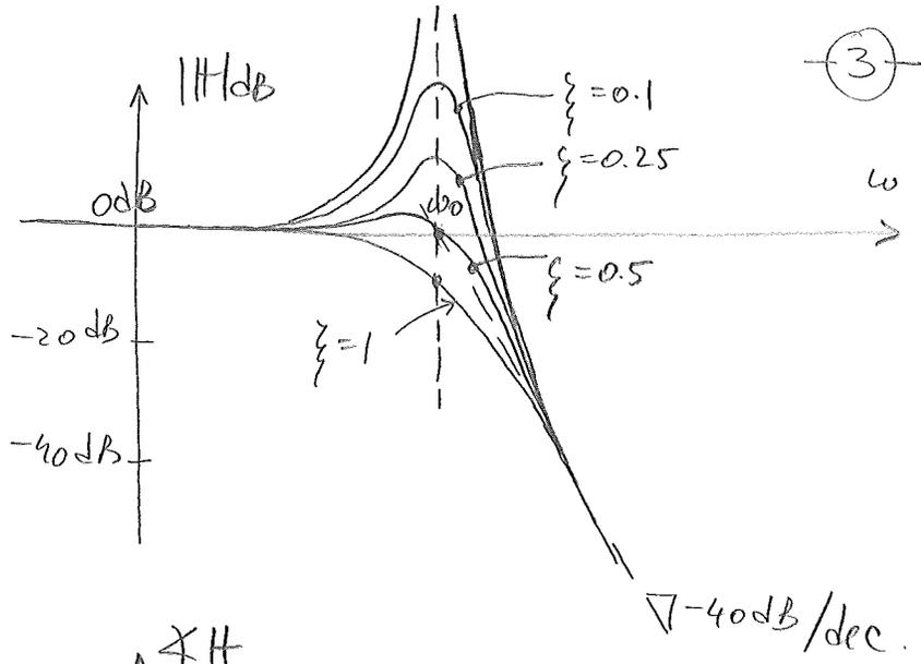
$$\left\{ \begin{array}{l} \omega \rightarrow 0 \\ \omega \ll \omega_0 \end{array} \Rightarrow \angle H(j\omega) = 0 \right.$$
