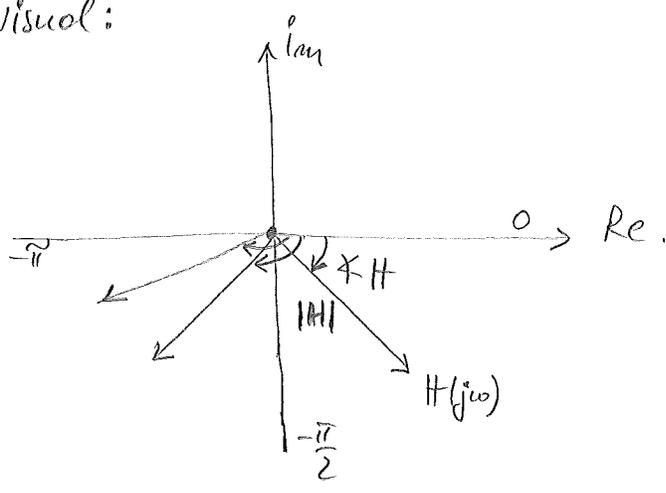
When  $\zeta \rightarrow 0 \Rightarrow |H| \rightarrow \infty \Rightarrow$  circuit capable of providing **ac** response even in the absence of any input signal!  $\Rightarrow$  sustained oscillation; poles are on imaginary axis  $\frac{s}{\omega_0} = \pm j$
