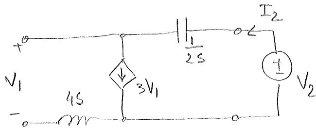
$$\left\{ \begin{array}{l} I_2 = 3V_1 \\ V_2 - V_1 = \frac{1}{2s} \cdot I_2 \end{array} \right| \Rightarrow \boxed{V_1 = \frac{2s}{2s+3} V_2} \text{ by } I_2 \text{ elimination} \\ \Rightarrow \boxed{I_2 = \frac{6s}{2s+3} V_2} \text{ by } V_1 \text{ elimination.}$$
