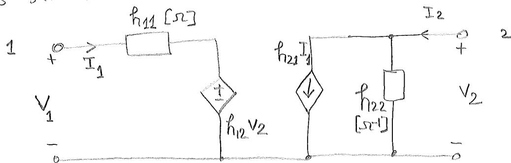
**Note :** This circuit is used to model the small-signal behavior of BJT's !
