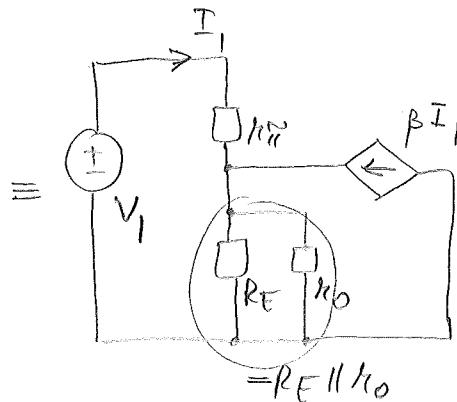
$$V_1 = r_{pi} \cdot I_1 + (R_E \parallel R_o) \cdot (I_1 + \beta I_1)$$
