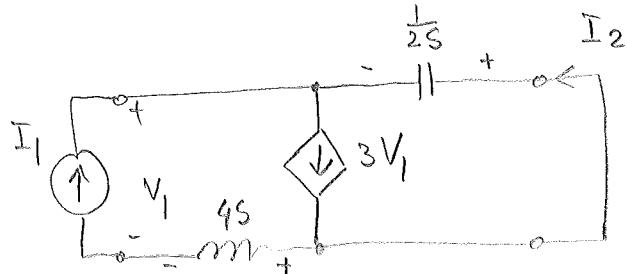
$$\text{KCL: } I_1 + I_2 = 3V_1$$
