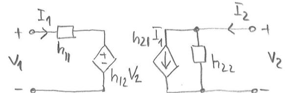
Voltage to voltage (or simply voltage) amplification:
