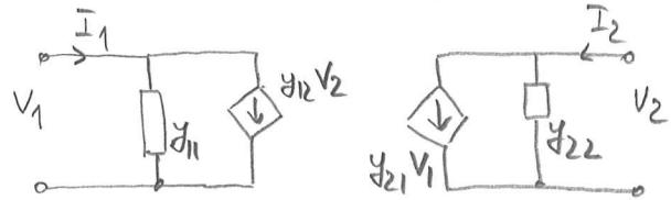
$$\left\{ \begin{array}{l} I_1 = y_{11}V_1 + y_{12}V_2 \\ I_2 = y_{21}V_1 + y_{22}V_2 \end{array} \right.$$
