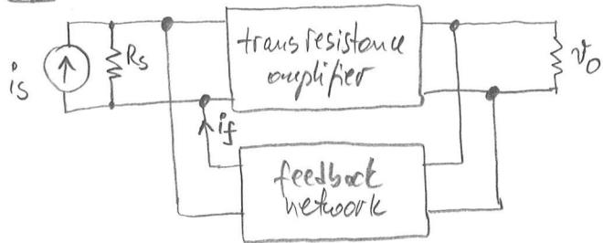
Current to voltage  $\Rightarrow$  transresistance amplifier (or converter).
