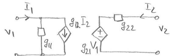
$$\left\{ \begin{array}{l} I_1 = g_{11}V_1 + g_{12}I_2 \\ I_2 = g_{21}V_1 + g_{22}I_2 \end{array} \right.$$
