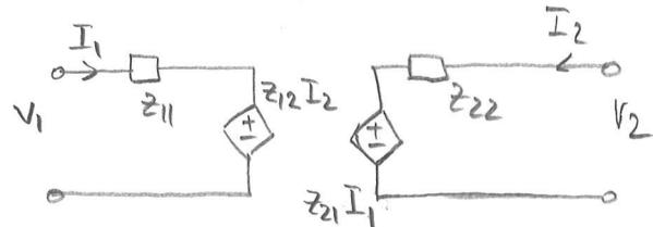
$$\begin{cases} V_1 = z_{11}I_1 + z_{12}I_2 \\ V_2 = z_{21}I_1 + z_{22}I_2 \end{cases}$$
