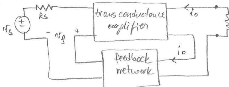
Voltage to current (or transconductance) amplifier (or converter).
