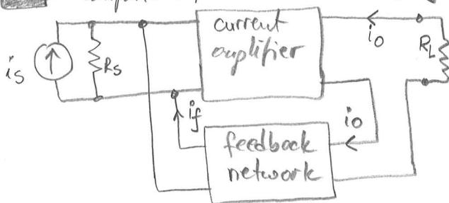
Current to current (or simply current) amplification:
