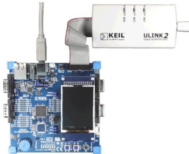
**Figure 1 Connection of ULINK2 to the board.**
