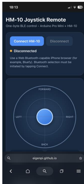
Figure 1: Online web joystick loaded on iPhone via Bluefy web browser.
