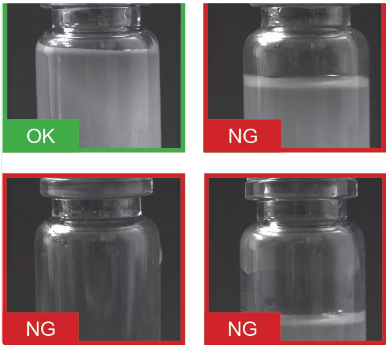
Figure 4: The transparent and reflective nature of both the glass vial and its contents makes it difficult for traditional machine vision to consistently detect the fill level.
