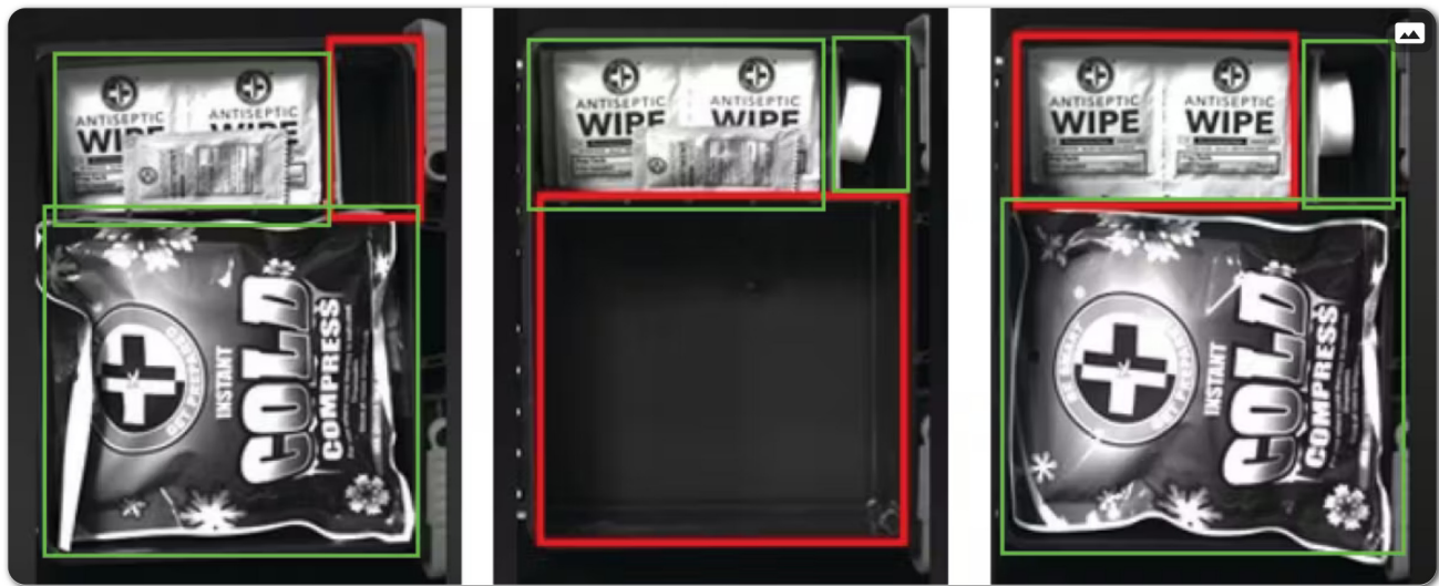
Figure 3: By performing multi-ROI assembly verification to check three different regions, edge learning tools can ensure that all necessary components are present in a first aid kit.
