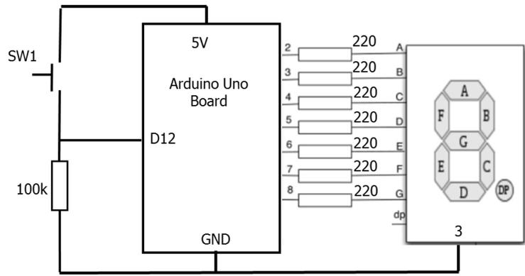
Figure 6: Schematic diagram of 3rd experiment.
