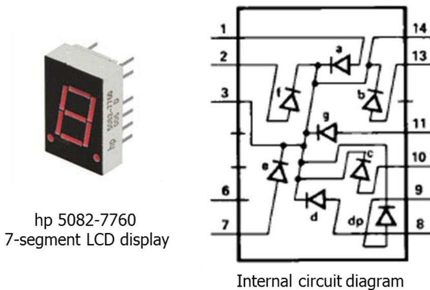
*Figure 5: Example of 7-segment LED display.*
