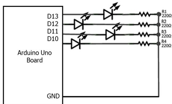
Figure 3: Schematic diagram of 2nd experiment.
