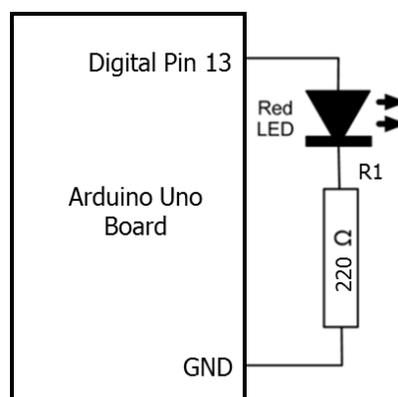
Figure 1: Schematic diagram of 1st experiment.
